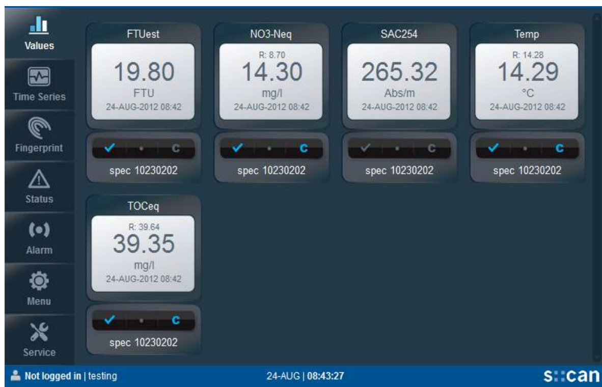
Photo. On-line transmission of selected data and presentation on a web page from the spectrometer S: Can Nitro: lyser, submerged in the river.
